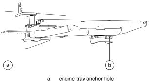
b engine tray retaining fastener
